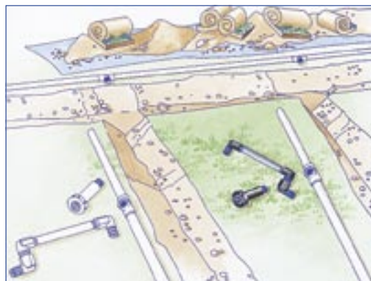
Lay out the pipes and sprinklers near the trenches where they will be installed.
